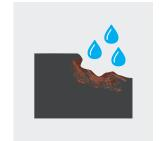
when drill holes and cut edges go through the galvanized plating to expose the underlying metal<sup>1</sup>.
